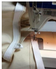
Figure 42 Webbing with loops being sewed to the top of the side wall
